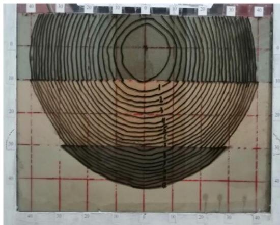
**Figure 7** The wetting front progress for a subsurface emitter in a stratified soil (sand, loamy sand, and silty clay loam),  $Q=1$  l/h,  $R=0.5$ , for 6 liters of water.
