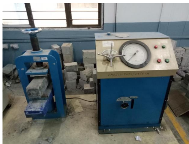
Fig. 3 Test setup for flexural rigidity
