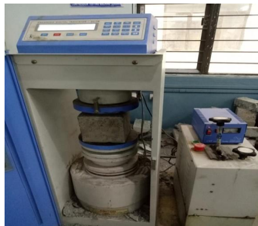
Fig. 2 Test setup for CTM
