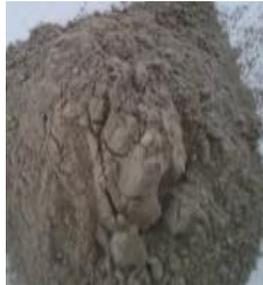
**Fig 2.** Photograph of Class C Fly-ash
