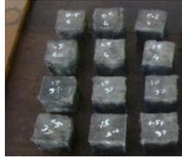
**Fig 4.** Ambient curing
