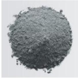
**Fig 1.** Photograph of Class F Fly-ash
