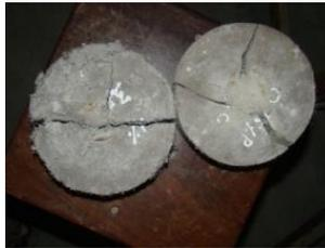
Fig 7. Crack pattern in the impact discs
