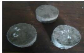
**Fig 5.** Specimens for drop weight impact test
