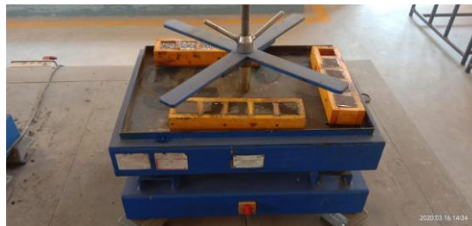
Fig 5: Compaction of mortar using vibrating table
