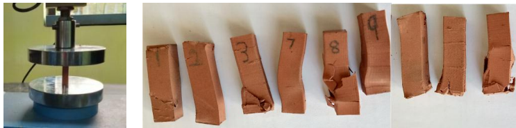
Figure 2 Experimental arrangements for compression test
