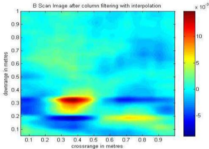
**Figure 18** B Scan Image of Cavity at Depth of 20 cm below Antenna After Interpolation
