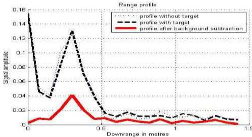
**Figure 14 A** – Scan of Water Buried 15 cm Below Sand Surface
