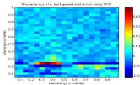
**Figure 16** B Scan Image of Cavity Buried 20 cm below the Antenna
