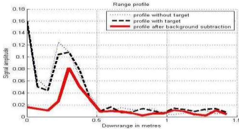
**Figure 13 A** – Scan of Water Buried 10 cm Below Sand Surface
