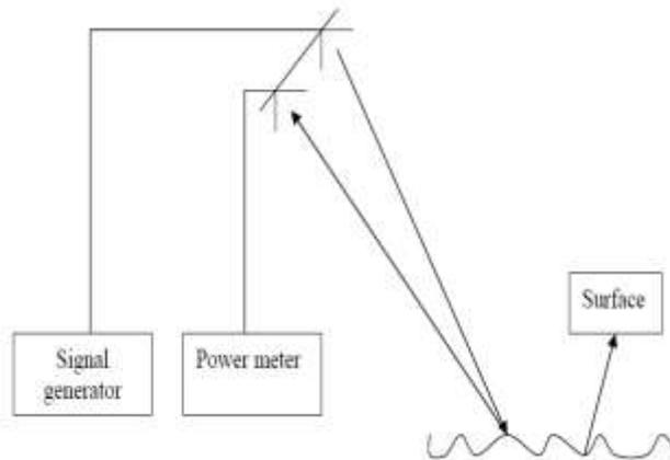
**Figure 1** Schematic of the Setup for Detection of Buried Object
