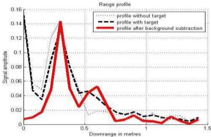
**Figure 9 A – Scan of Cavital Buried 5 cm Below Surface**
