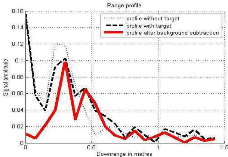
**Figure 10 A – Scan of Cavital Buried 10 cm Below Surface**
