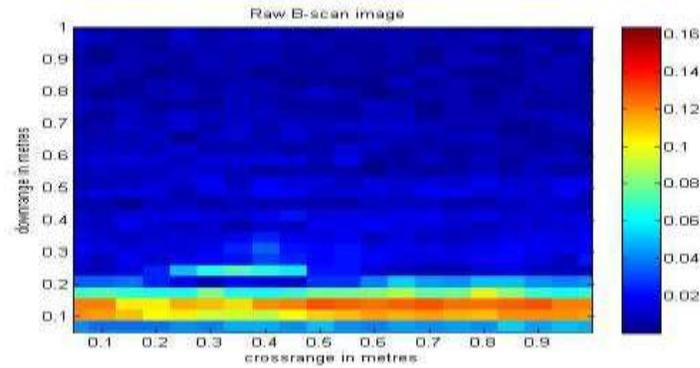
**Figure 15** B Scan Image of Cavity Buried 20 cm below the Antenna
