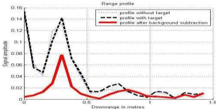
**Figure 12 A** – Scan of Water Buried 5 cm Below Sand Surface
