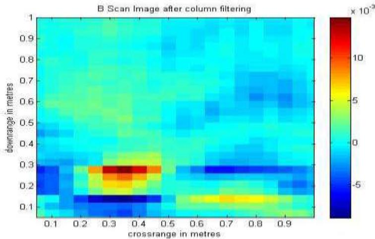
**Figure 17** B Scan Image of Cavity at Depth of 20 cm below Antenna after Column Filtering
