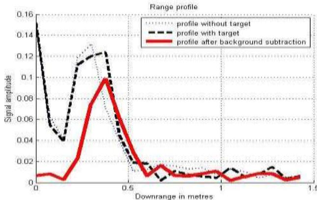
**Figure 9** A – Scan of metal buried 15 cm below surface
