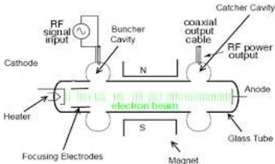
**Figure 2** Internal Block of Two Cavity Klystron Amplifier.
