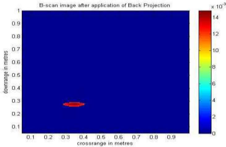
**Figure 19** B Scan Image of Cavity Buried 20 cm below Antenna after Back-Projection
