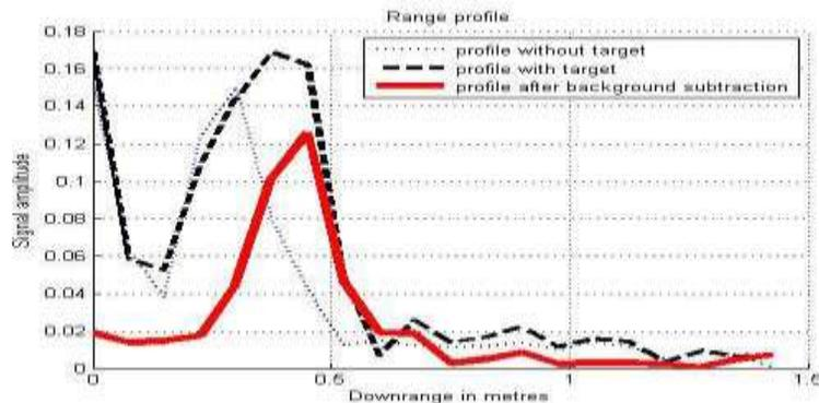
**Figure 7** A Scan of Metal Buried 5 cm Below Surface
