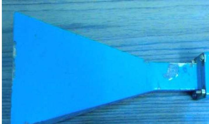
**Figure 3** Top View of X Band Horn Antenna used
