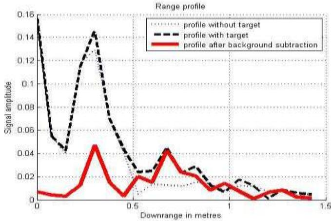
**Figure 11 A** – Scan of Cavity Buried 15 cm Below Surface
