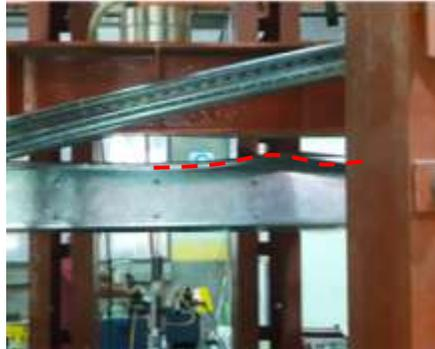
**Figure 11** Development of wave pattern for SAFT-07
