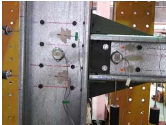
**Figure 4** Installed specimens of IJT inside frame rig
