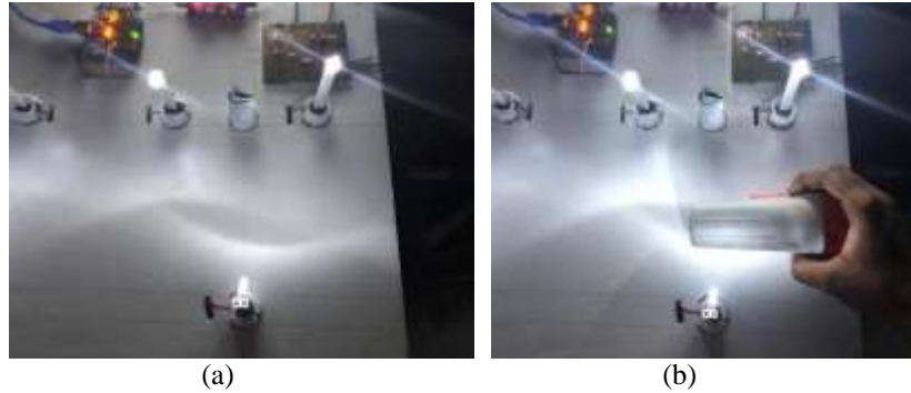
Figure 6 Motion detection by PIR sensor (a) light intensity is 50% and (b) light intensity is 100%
