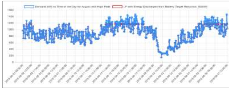
Figure 2 Load Demand Analysis for a Typical Industrial Customer after BESS Installation
